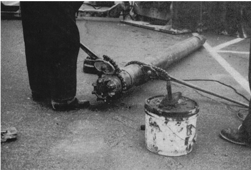
Figure 3-8. Photograph of a plugged bit which is used to obtain Becker penetration resistance (Harder 1993)
