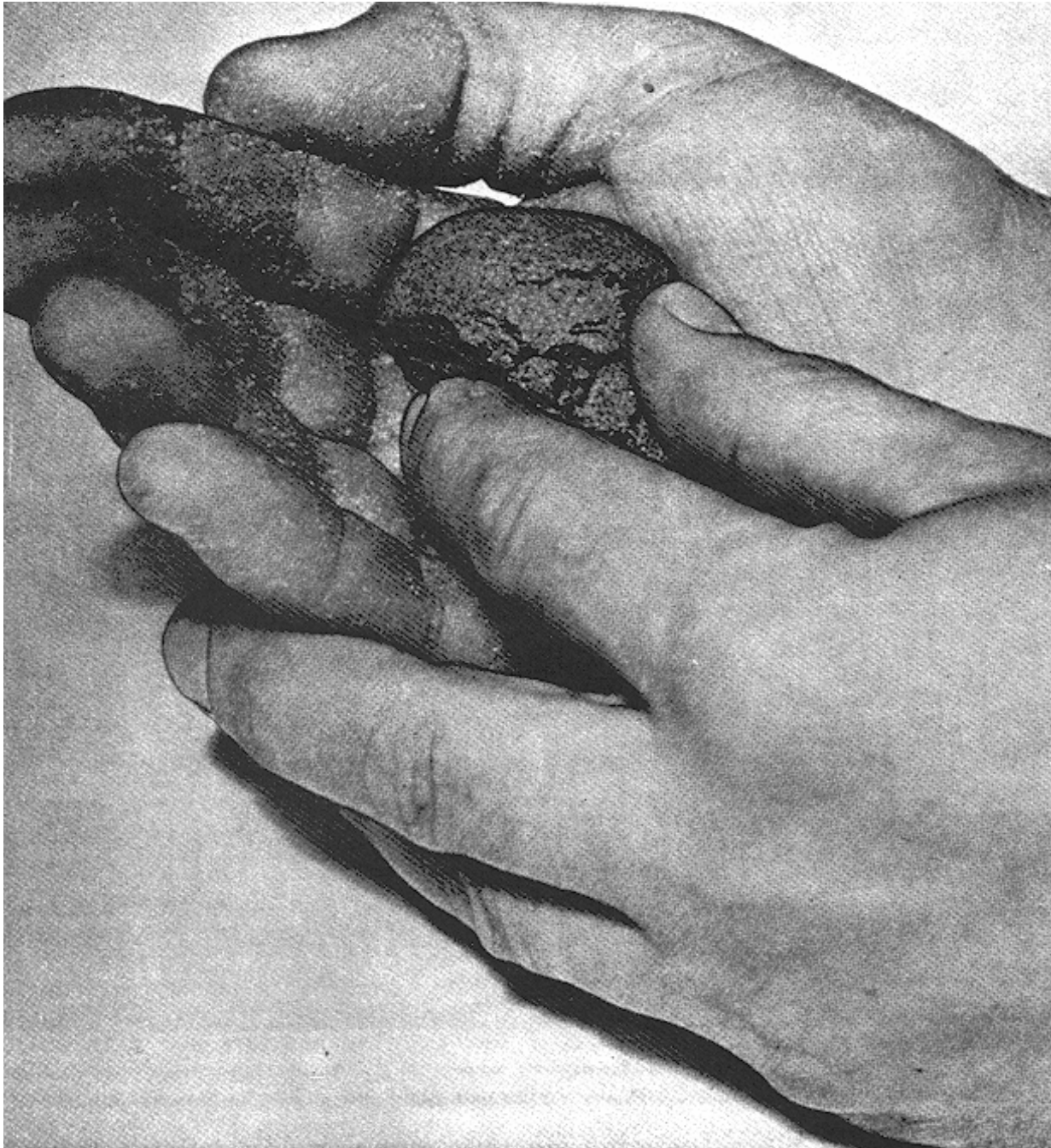
Figure E-7. A sample of a moist, fine-grained soil cracking and crumbling during the dilatancy test
