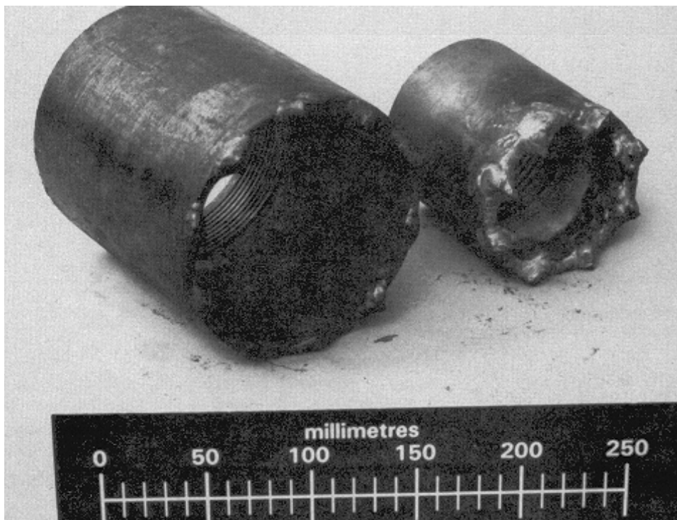
Figure 3-17. Photograph of a standard carbide insert bit and a pyramid carbide bit
