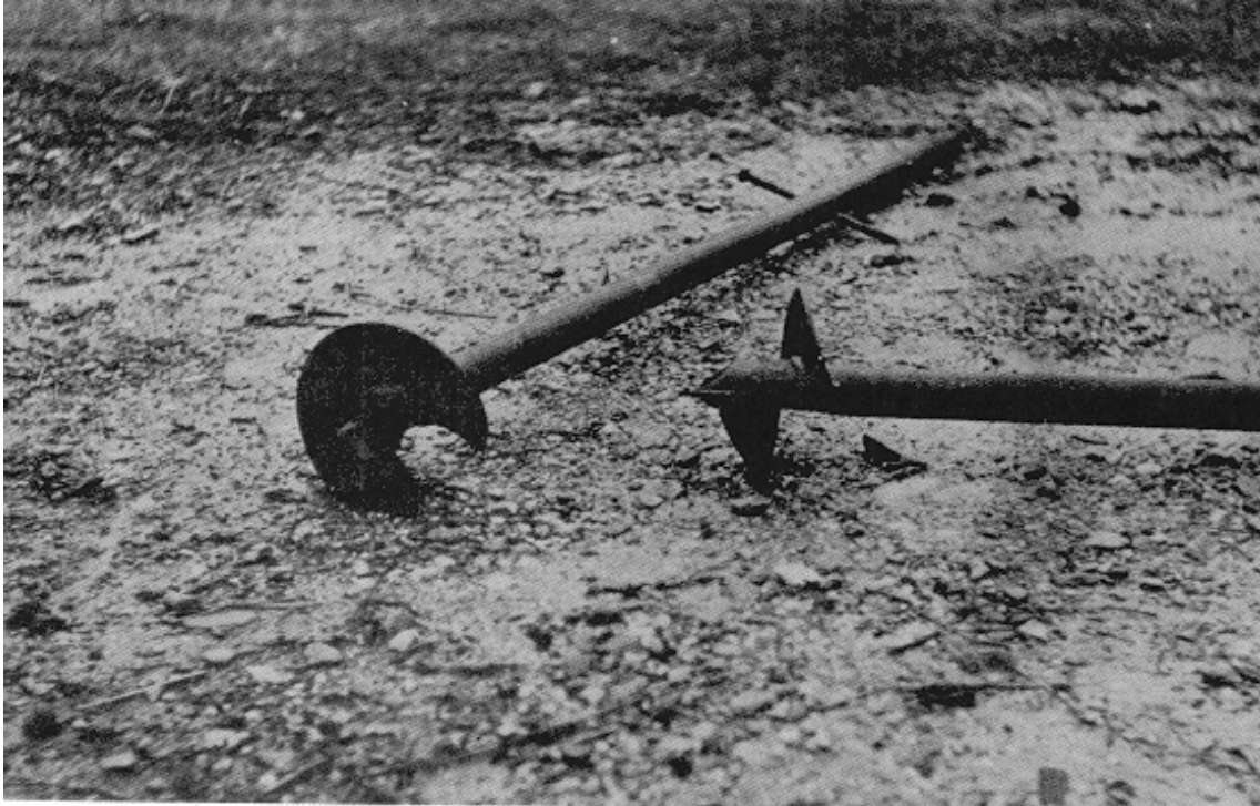
Figure 6-1. Photograph of screw-type earth anchors
