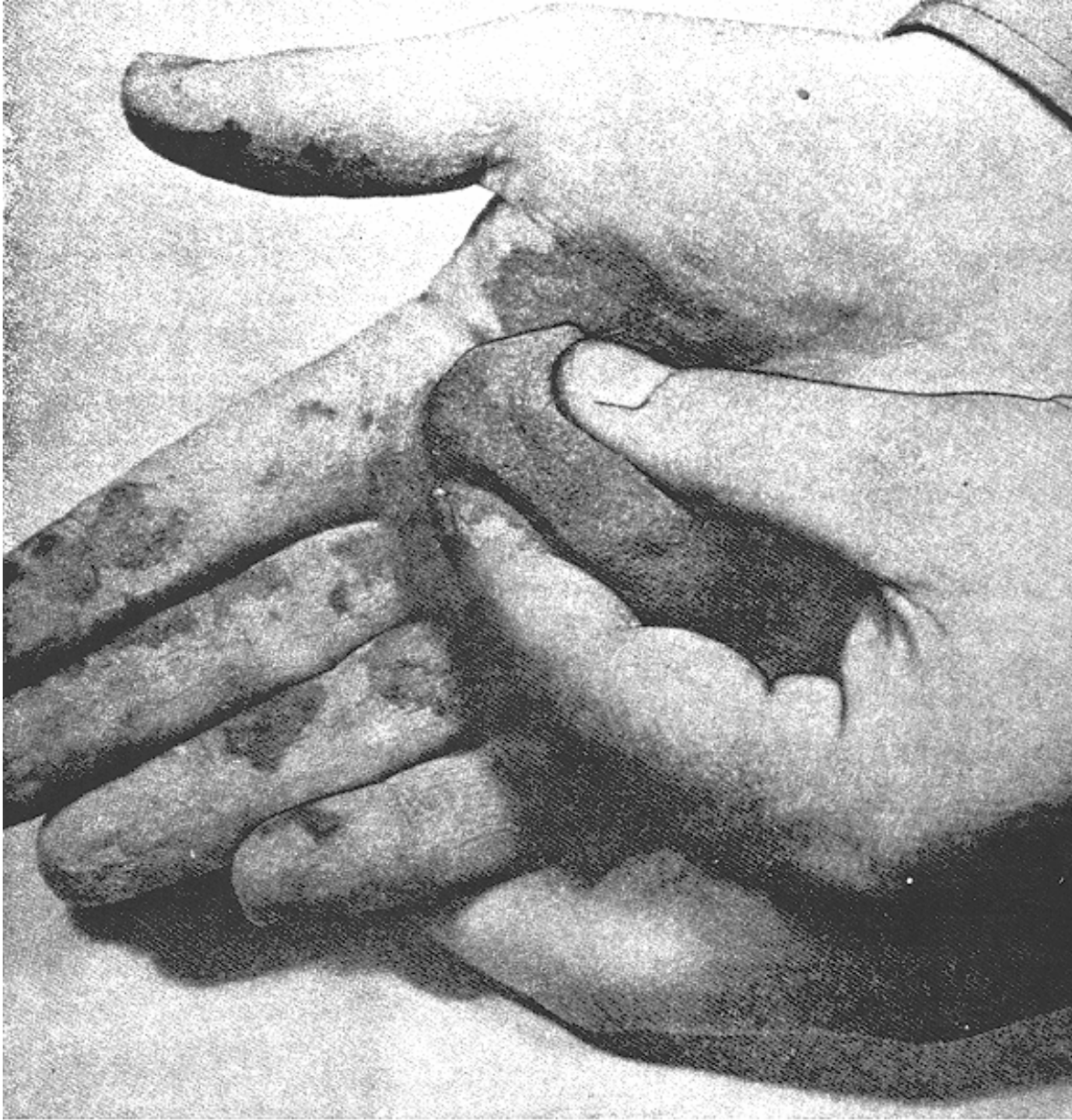
Figure E-6. Photograph of a sample of a moist, fine-grained soil being squeezed during the dilatancy test
