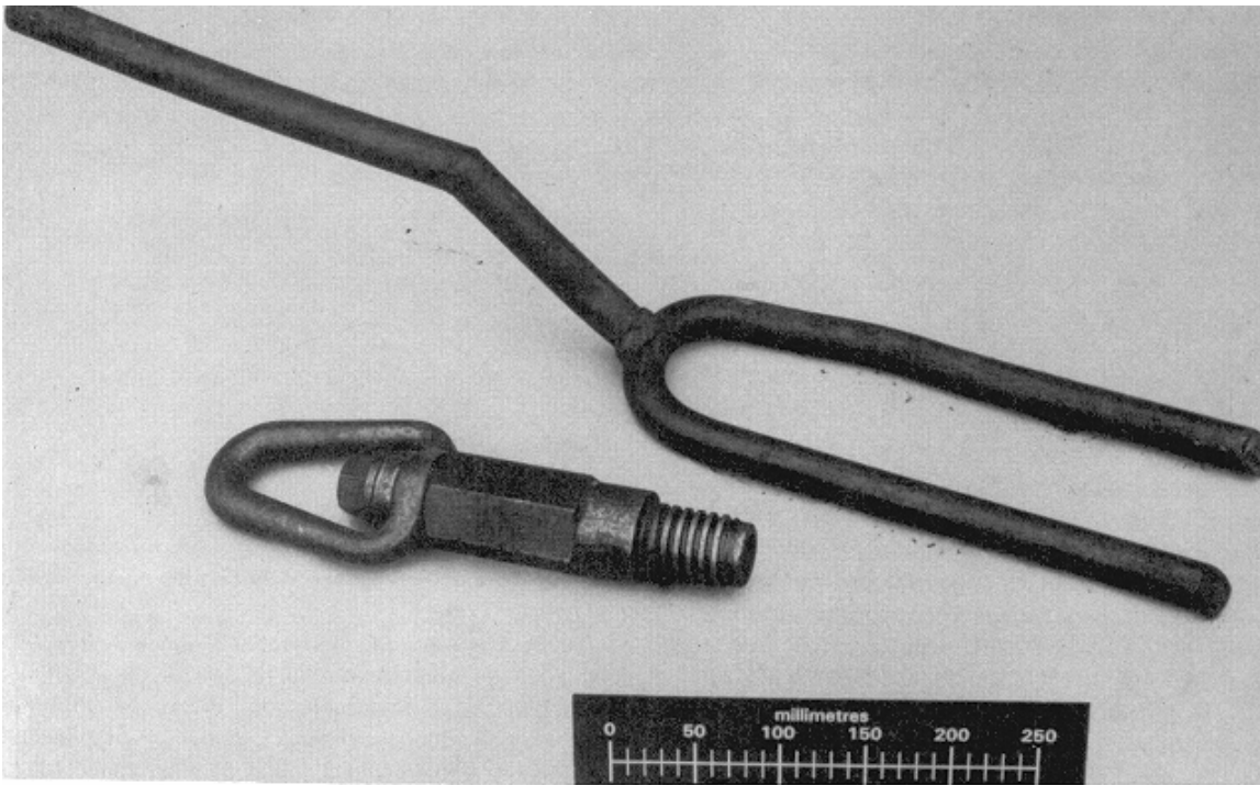
Figure 3-19. Photograph of a holding fork and a hoisting plug
