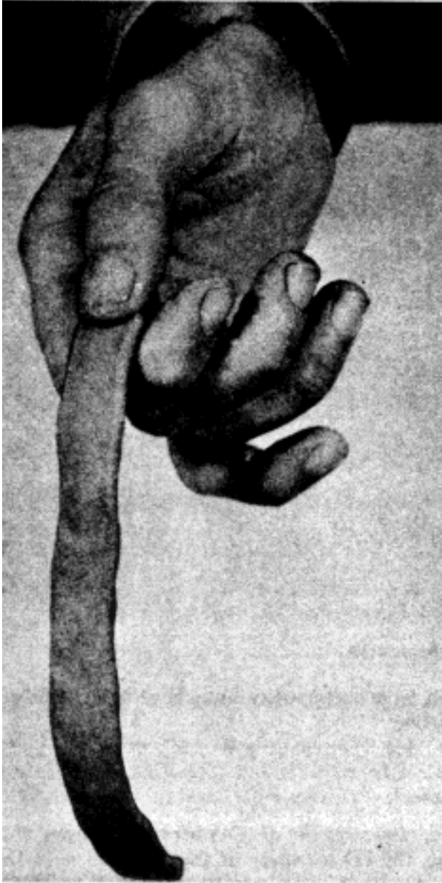
Figure E-10. Photograph of a sample of a moist, fine-grained soil being flattened to a ribbon about 3 to 6 mm (1/8 to 1/4 in.) thick to determine its toughness and plasticity
