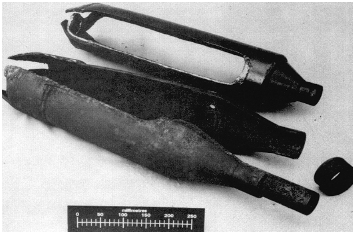
Figure 7-2. Photograph of the Vicksburg solid and hinged barrel-type augers
