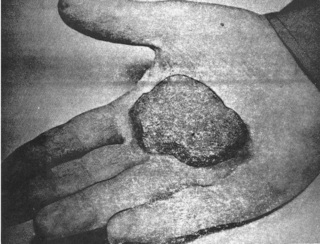
Figure E-4. Appearance of a sample of moist, fine-grained soil prior to conducting the dilatancy test.
